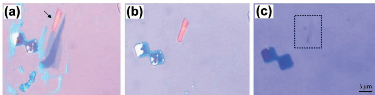
Figure 3. Optical images of MHA-masked monolayer graphene (pink area indicated by an arrow) after (a) Au etching, (b) O 2 plasma etching of exposed graphene layers, and (c) Au etching to reveal the protected flake within the dotted black rectangle. The pairs of blue squares are alignment markers.
